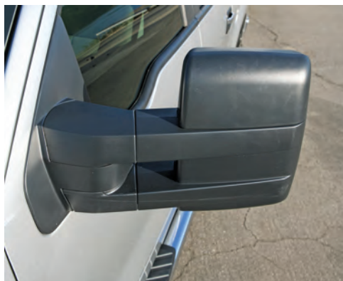
Ford's towing mirrors easily extend for optimum visibility of the trailer.
